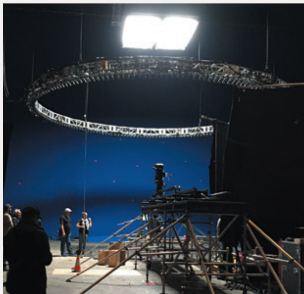
The Satellite Lab team programmed the lighting array so that each sequential strobe was synced to a sequential frame in the Phantom camera.
